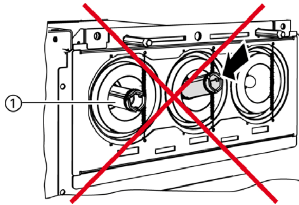
Fig. 116: Incorrectly inserted contact coupling
