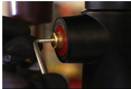
Figure 2: The capacitive test plug inserted until flush with the connector body
