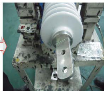
Check to ensure the terminal palm is horizontal, if not, gently rotate it to bring it into the horizontal plane. Do not rotate more than about 20-30° to bring it into the correct position.
