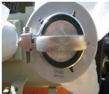
Bring the two sides of the clamp together using multi grips, vice grips or a similar tool. Once the two sides are close enough together insert the bolt and tighten.
