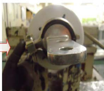
Tighten the clamp using the bolt so the top and bottom halves of the clamp come together.
