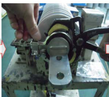
Bring the two sides of the clamp together using multi grips, vice grips or a similar tool. Once the two sides are close enough together insert the bolt and tighten.
