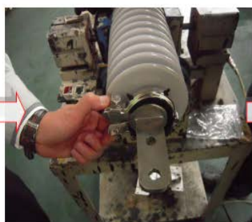
Fit clamp to bush and terminal palm
