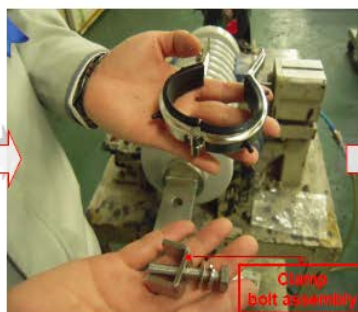
Unscrew the bolt from the clamp so it come open.
