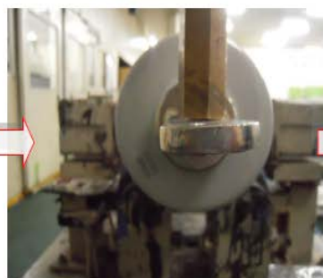
Rotate the terminal palm, if required to bring into the correct horizontal plane. You will notice there is a thick section and a thin section to the EPDM packing on the clamp assembly
