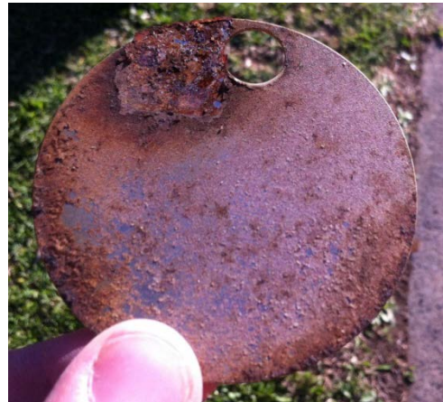
Figure 2 – Semaphore cover corroded off
