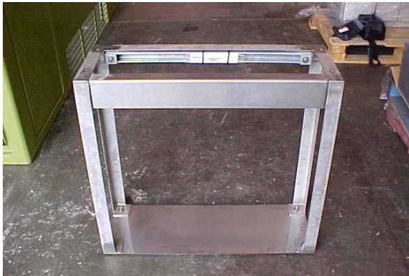
Figure 25: Stainless steel mounting frame
