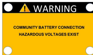
Figure 3: Warning label to be applied to switch pillar and supplying distribution substation.
