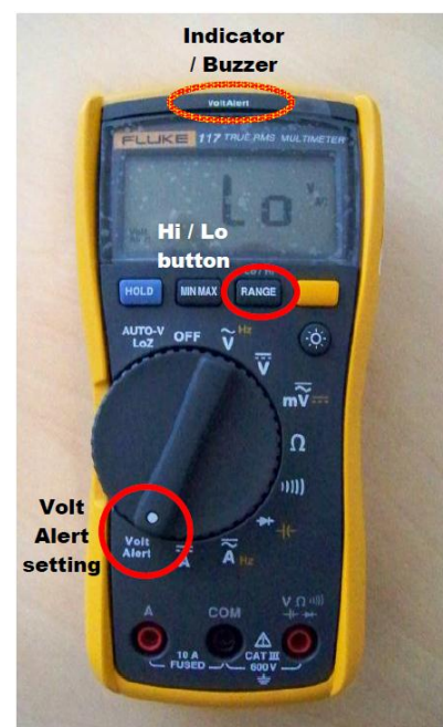
Figure 1 - Settings for multimeter check and high impedance check
