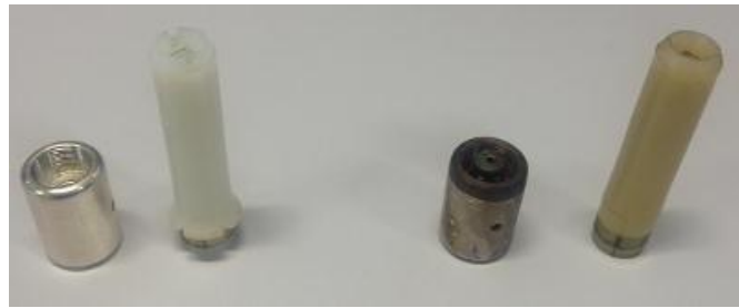
Figure 7-16: New (left) and old (right) arcing chambers
