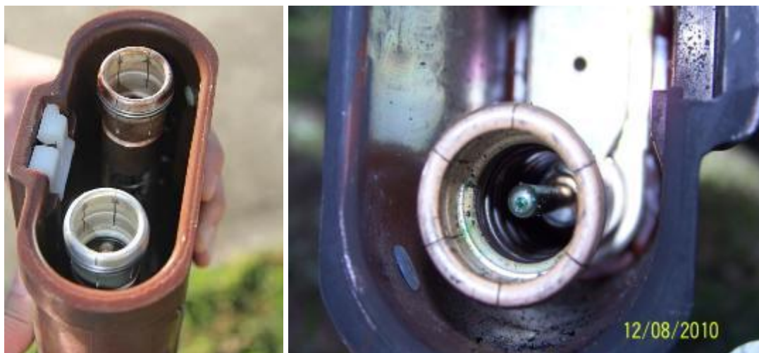
Figure 7-11: Discolouration of moving main contact
