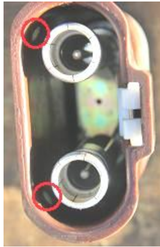
Figure 7-33: Location of the mounting screws
