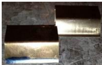
Figure 7-4: Three phase (blue) and single phase leaf springs
