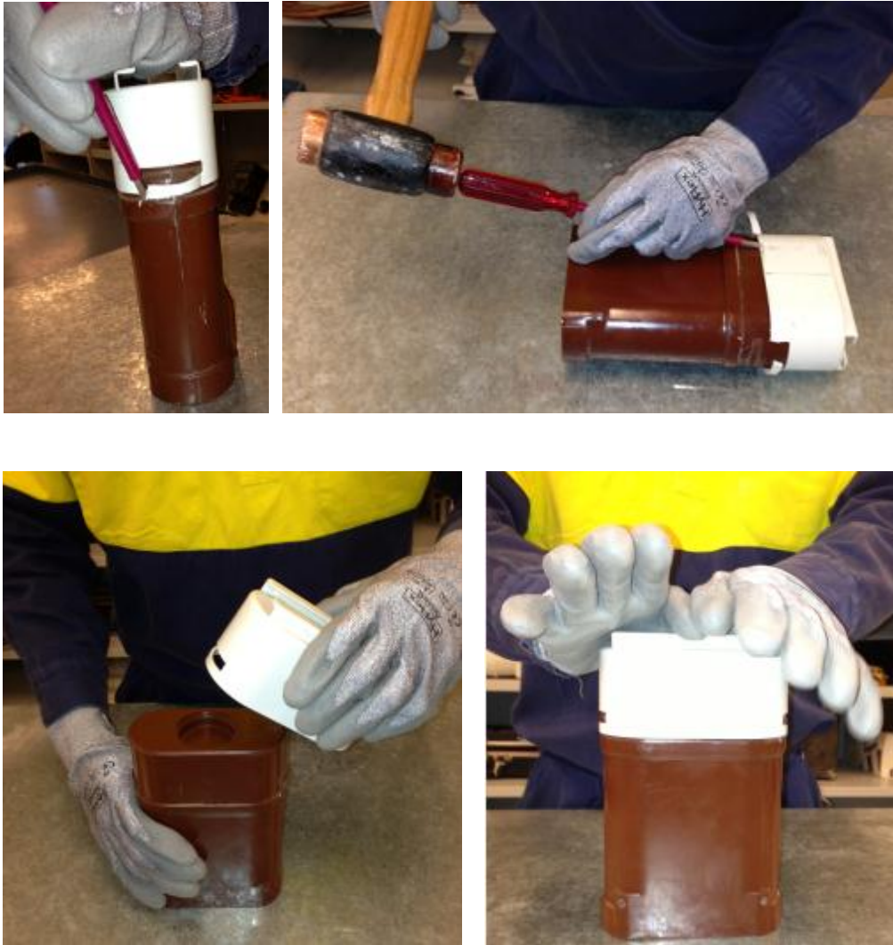
Figure 7-31: Procedure to replace a protective cap
