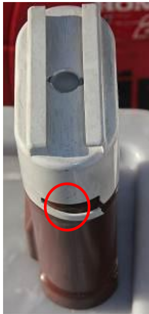
Figure 7-30: a) Cracked protective cap
