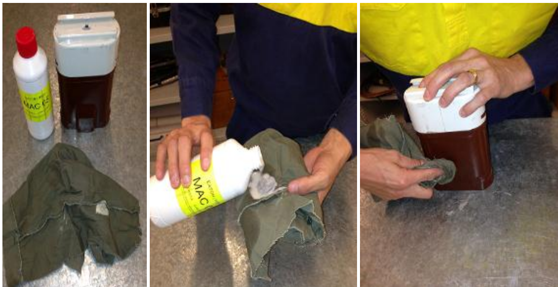
Figure 7-34: Applying cleaning agent to the outside of the switch cap
