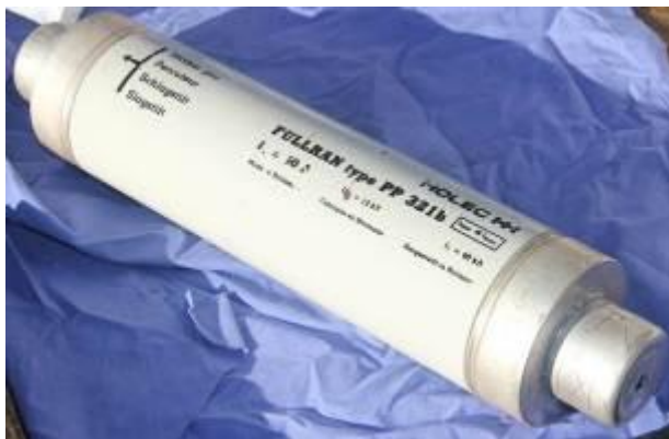
Figure 7-27: Fuse before cleaning
