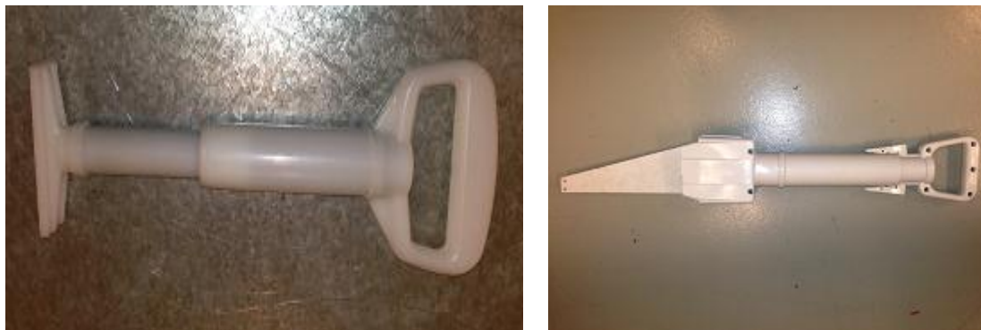
Figure 7-7: a) Single phase and b) Three phase operating handles
