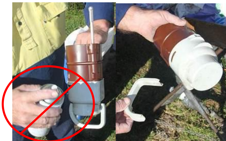
Figure 7-26: How CRC NF 2017 contact cleaner damages fuse cap handle
