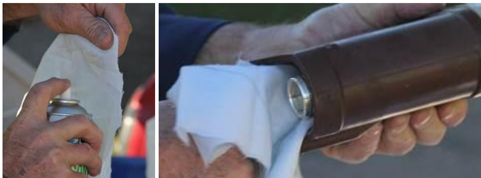
Figure 7-35: Cleaning the main contacts
